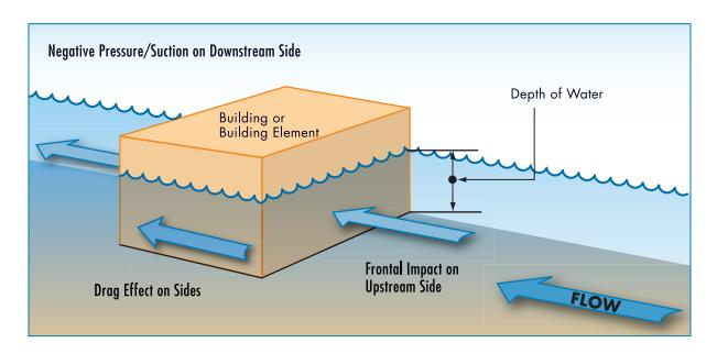
Figure 2-9: Hydrodynamic loads on a building or building element
