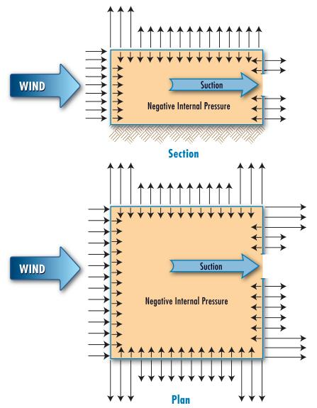
Figure 3-7: Schematic of internal pressure condition when the dominant opening is in the leeward wall
