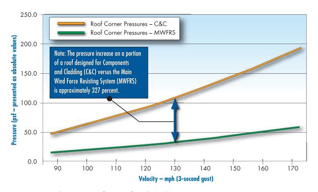
Figure 3-5: Wind pressure as a function of wind speed
