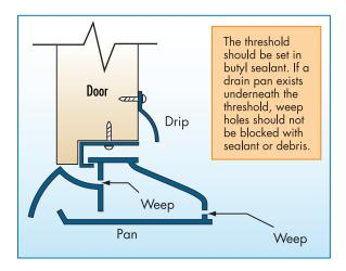
Figure 3-35: Interlocking threshold with drain pan
