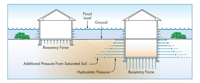
Figure 2-8: Hydrostatic loads on buildings
