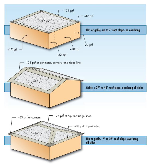
**NOTE:** Design pressures all assume an enclosed building with the same basic wind speed of 90 mph, Exposure B, 30' roof height, and an importance factor of 1.15
