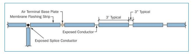
Figure 3-98: Plan showing conductor attachment
