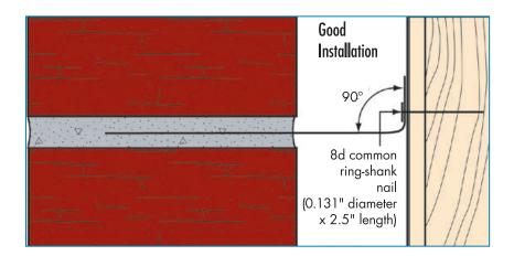
Figure 3-50: Bend ties at nail heads
