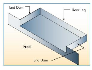
Figure 3-39: View of a typical window sill pan flashing with end dams and rear legs
