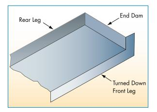
Figure 3-31: Door sill pan flashing with end dams, rear leg, and turned-down front leg
