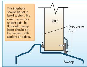
Figure 3-36: Threshold with stop and seal
