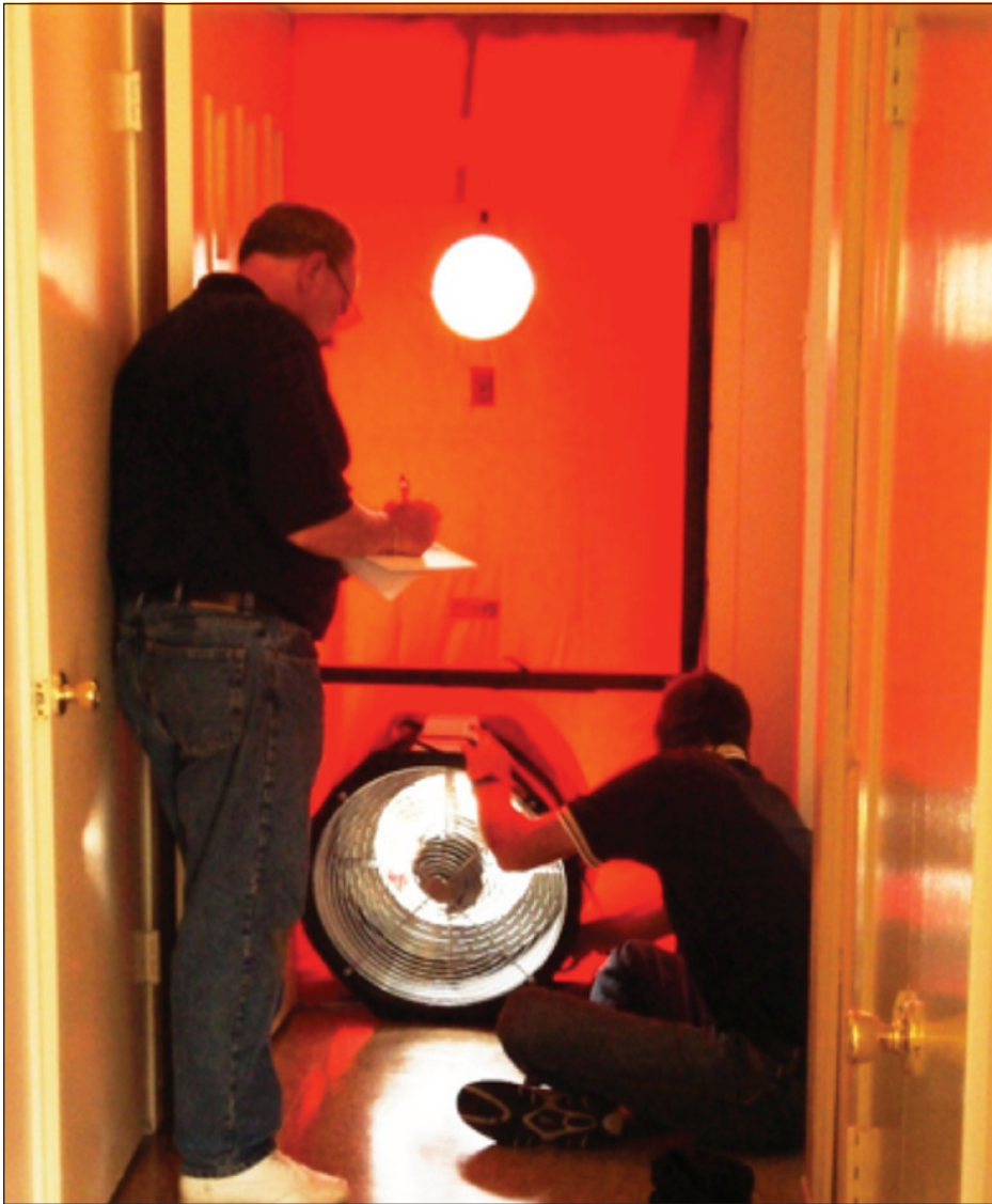
Figure 4-6: Blower door testing
