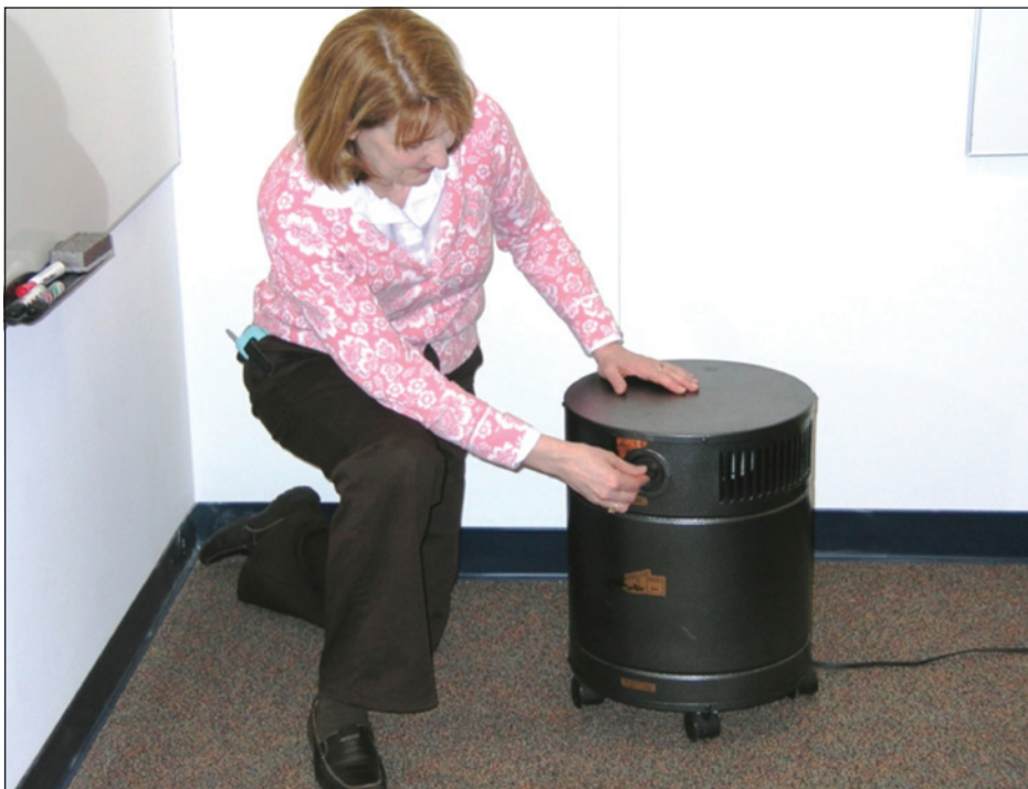
Figure 4-12: A portable, floor recirculation filter unit with an adsorber and HEPA filter
